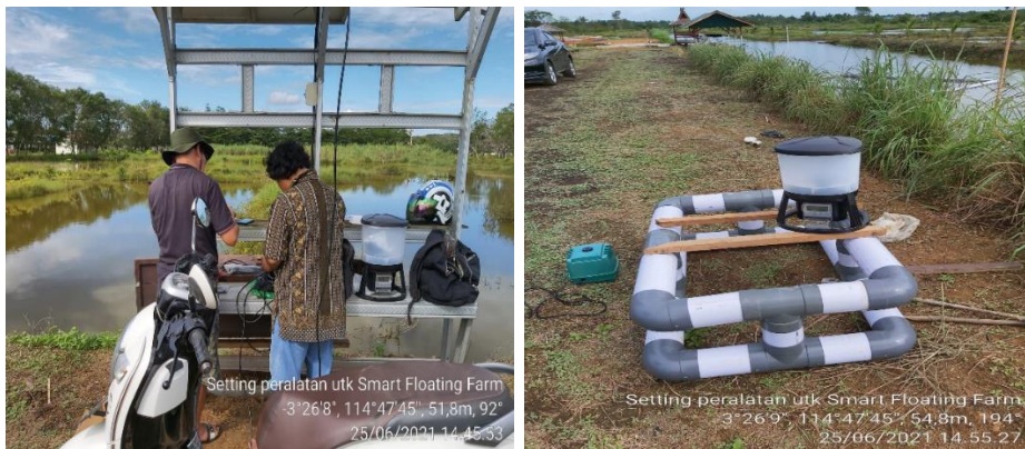
Gambar 57. Setting peralatan automatic fish feed , digital timer, dan aerator
